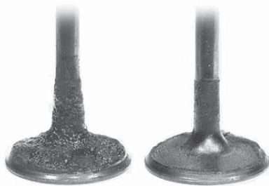
Intake valve before P.i. treatment.
