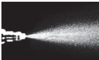
Injector spray pattern after P.i. treatment.
